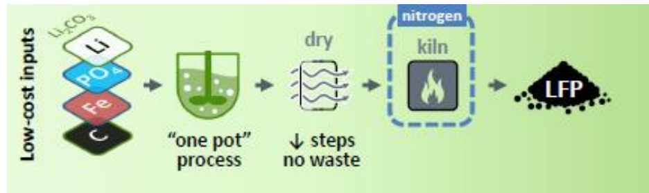
Figure 9: Nano One LFP Process
